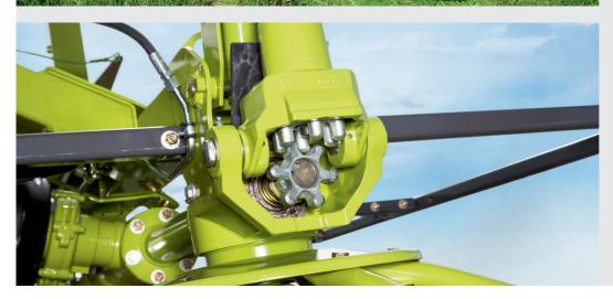
PERMALINK connection provides positive drive and allows the outer rotors to fold up 180° for transport.
