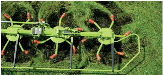
Spreader arms angled at 29° on the VOLTO 55 produce a wider, more even spread pattern with fewer lumps promoting faster, uniform drying.
