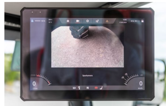
High-resolution, individual display of the track camera in the A-column display
