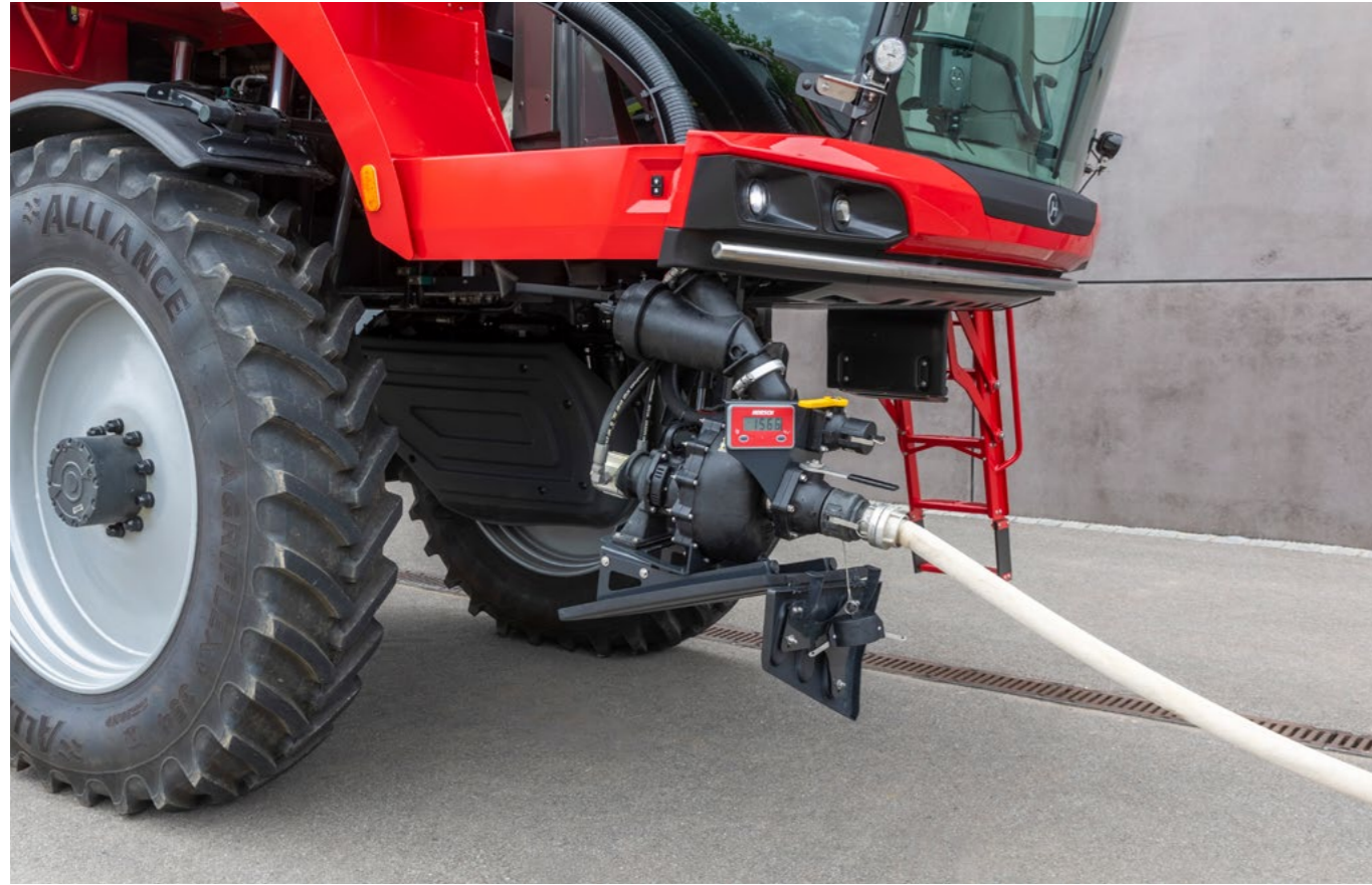
PowerFill filling pump with 1 000 l/min capacity – 3" Camlock filling connection in the front
