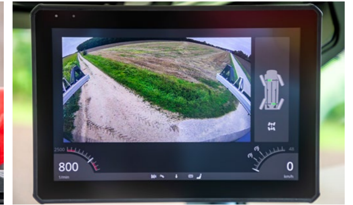
High-resolution, automatic display of the rearview camera in the A-column display
