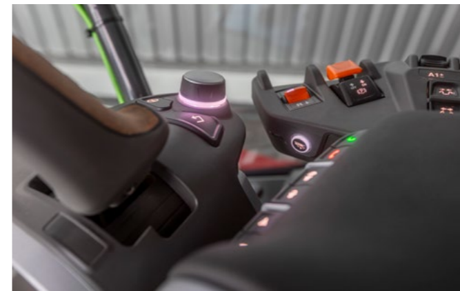
Safe operation of the A-column display: rotary/push functions
