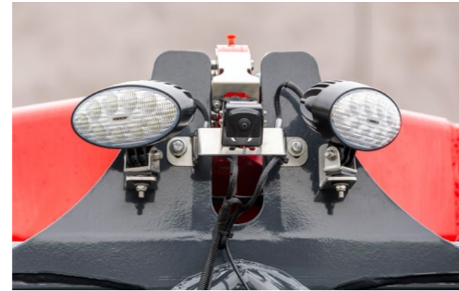
Rear view camera for monitoring the area behind the vehicle
