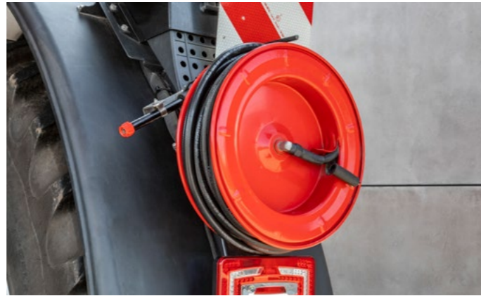
Hose drum for outside cleaning
