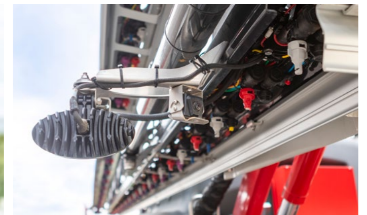
Camera for nozzle monitoring on the NightLight holder
