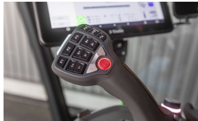
Ergonomic control lever with multiply assignable buttons
