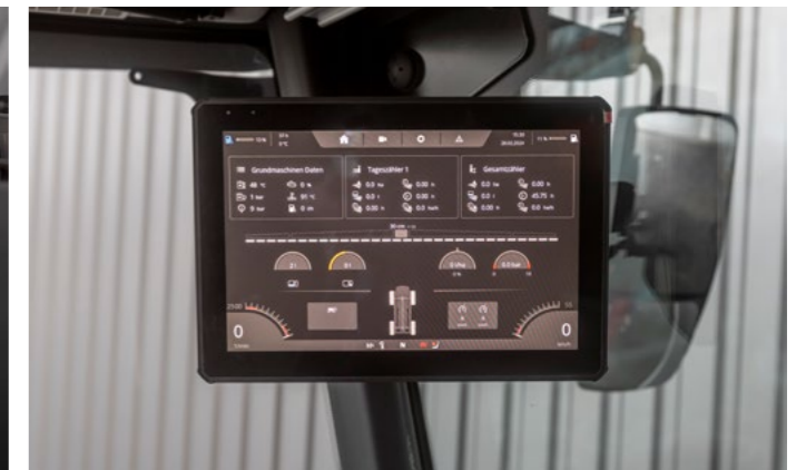
Standard 12" A-column display with freely assignable display
