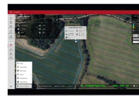
Success factor transparency: position-specific data of all relevant information like error messages, application rate, nozzle status or target area spacing
