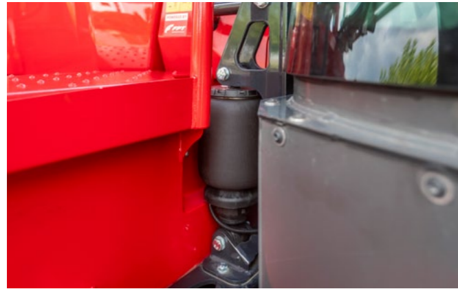
Pneumatic 4-point cabin suspension
