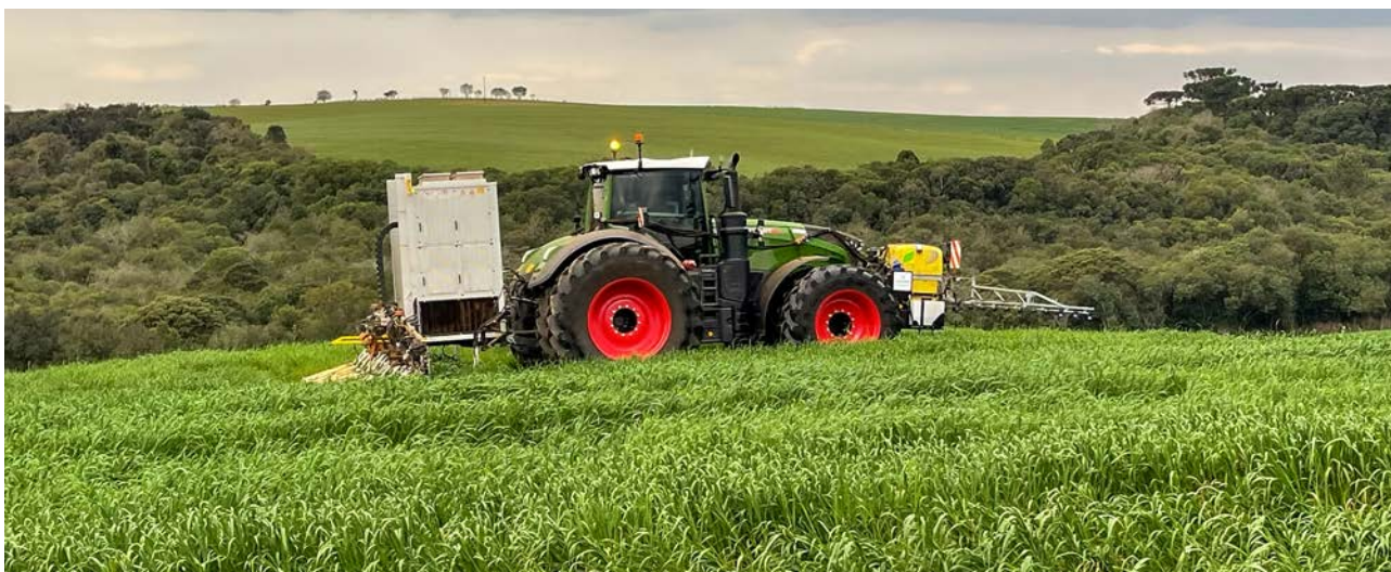
Catch crop killing for direct seeding in tests in Brazil with electricity in combination with a salt solution that was applied in advance to increase conductivity on the plant.
