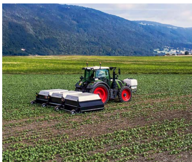
Ecorobotix offers an application device that achieves a stable detection by means of a hermetically shielded area.
