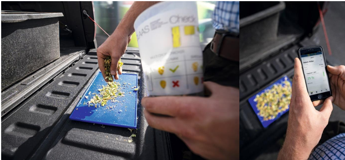
What previously required a laboratory can now be done directly in the field during the harvest: Determining processing intensity using the app in the new CLAAS connect.
