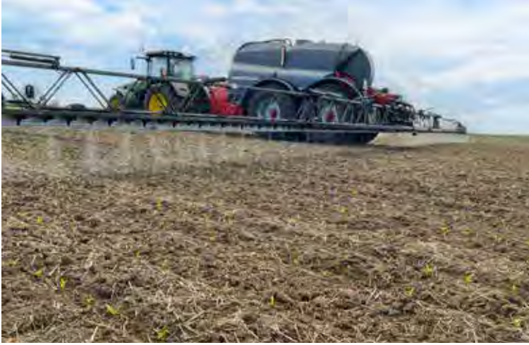
Herbicide application as strip spraying in sugar beet with a row width of 45 cm carried out by a HORSCH Leeb 12 TD.
