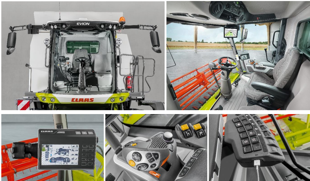
Control and monitoring of all key functions with CEMIS 700, CMOTION and multifunction armrest, with CEMIS 1200 interface for automated steering using GPS.
