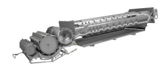
The operator has greater control over the threshing area. The main concave flaps can be engaged hydraulically from the cab and there is a new hydraulic pivoting concave bar between the preseparation concave and main concave that can be engaged via CEBIS in harder to thresh crops. Again the concaves are infinitely adjustable in CEBIS and fully integrated into AUTO CROP FLOW and CEMOS AUTOMATIC.
