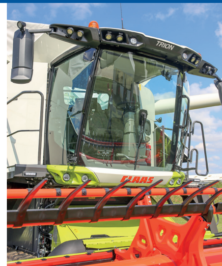
The threshing, separation and cleaning systems are all upgraded, and the cab is larger and more comfortable.
