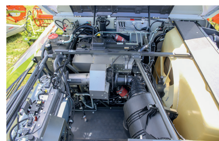
New British-built Cummins 6-cyl engines with 6.7- or 8.9-litres capacity power the new combines. Dynamic Power is standard across all models – providing significant fuel savings by producing only as much power as required.
