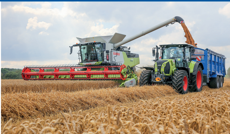
Larger tank capacities from 8,000–12,000 litres are available depending on model, with unloading rates up to 130 litres/second. An optional pivoting spout controlled from the C-Motion joystick helps achieve accurate trailer filling and offers particular advantages when unloading on slopes.
