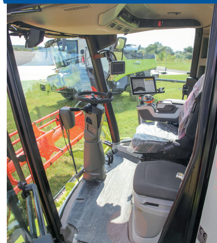
The new cab has more head and legroom, and a larger windscreen. The door is all glass and higher than before, improving the view for unloading. Other improvements include a swivelling seat, and extra functions for the Cebis 12in terminal including Cemos Dialog or Cemos Automatic when fitted.
