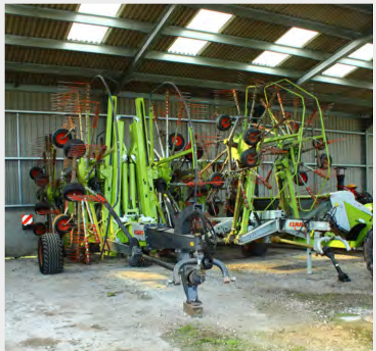
Notice the difference in transport height between the new LINER 4800 (left) and the 3500 beside it.
