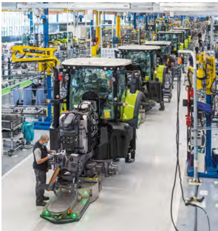
The traditional production line has been replaced with automated guided vehicles (AGV) at the new Le Mans factory.
