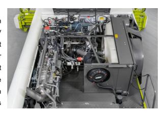
As standard, all TRION models come with DYNAMIC POWER, which by reducing engine power output when not under load, for instance when not running the chopper or unloading, can cut fuel costs by around 10%. The rated engine speed is just 1,900rpm dropping to 1,650 for road travel, so further helping to save fuel.
