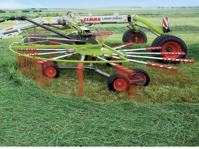
• 3D rotor suspension follows ground contour for clean swath. • Oil immersed cam track for continuous lubrication. • PROFIX tine arms for easy removal and strength.\* • Manual or electro-hydraulic raking height adjustment for easy setup. • Visible raking height guide gives clear view from tractor cab. • Jet effect rotor lift and lowering for clean raking. • 4 and 6 wheel rotor carriage for excellent ground contour following. • Pre determined bend on tine arms reduces damage.
