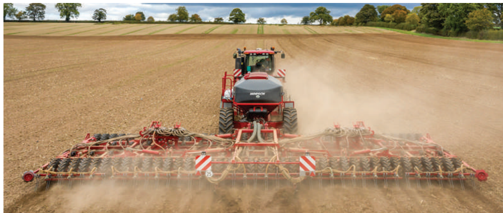
Variable rate and grain & fertiliser is used with Barton Farm’s Sprinter 12 SW (Image from Pro Horizon)
