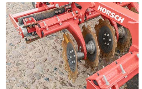
Having two discs on each leg helps to create some extra soil and trash clearance.
