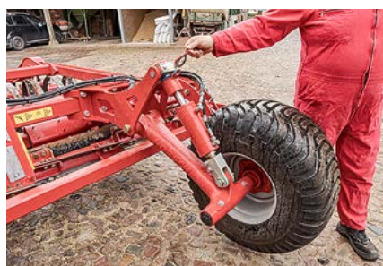
Levelling is done using clip-on shims. The working depth is controlled hydraulically on the full-spec machine.
