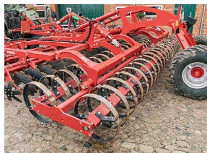
Our machine's rear roller is suspended from its mid-point, allowing it to adapt front to back. The roller coped well with different depths.
