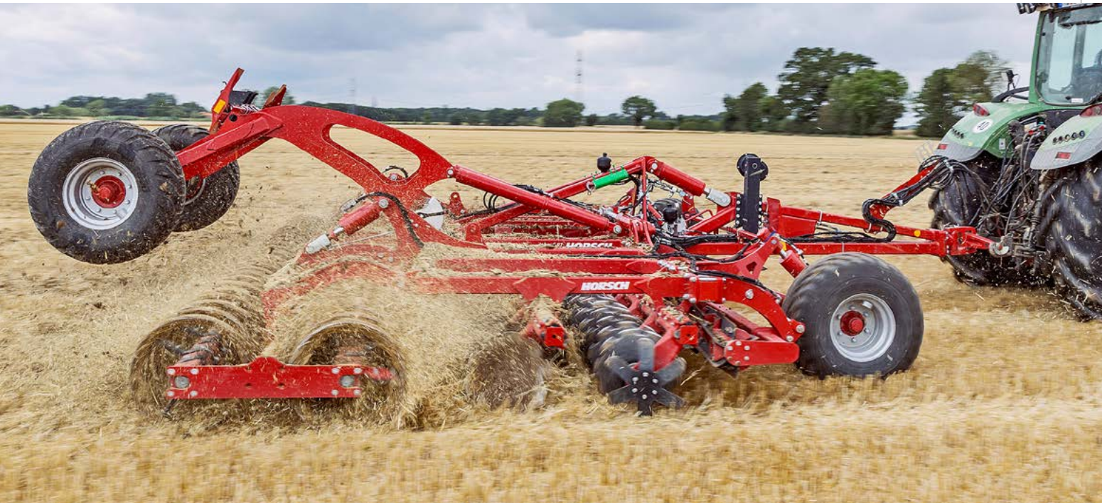
The Joker RT is the Horsch semi-mounted trailed disc harrow, slotting in above the CT mounted range with the same disc arrangement.
