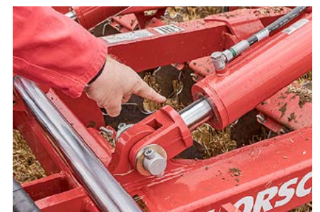
Clips have to be inserted to secure the machine in its transport position – not convenient.
