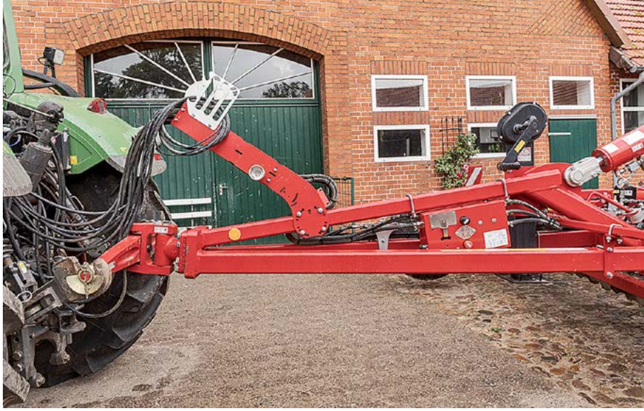
The drawbar has come out well – from the offset pivot point to the hose rack and parking stand.
