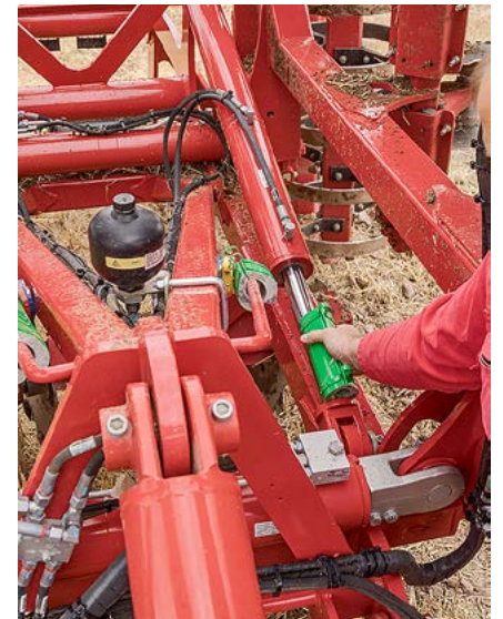
When not fully retracted, an accumulator cushions the chassis in the field.
