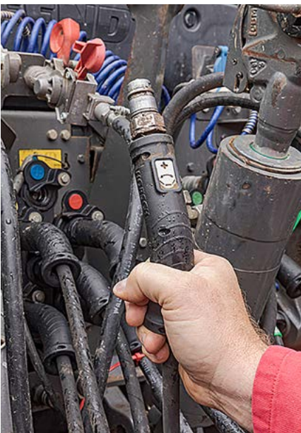
The angled oil couplers, with pictogram for identifying their function, are great.
