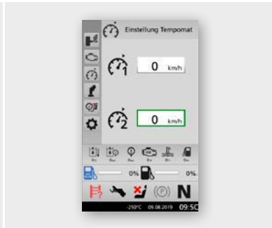
Two speed controls can be saved with an accuracy of 0.1 km/h
