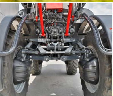
Underbody cover and fairing of the wheel motors protect the population
