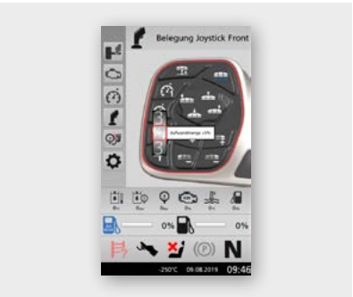
The function of freely configurable keys on the joystick of the ErgoControl can be selected via the vehicle display
