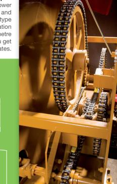
Big rotor for high throughput A rugged chain drive is used to power the large diameter spreading rotor and the hydraulically operated guillotine type side door allows you to control application rates. The SDS has a massive 1.5 metre wide spreading rotor which means you get high throughput rates.
