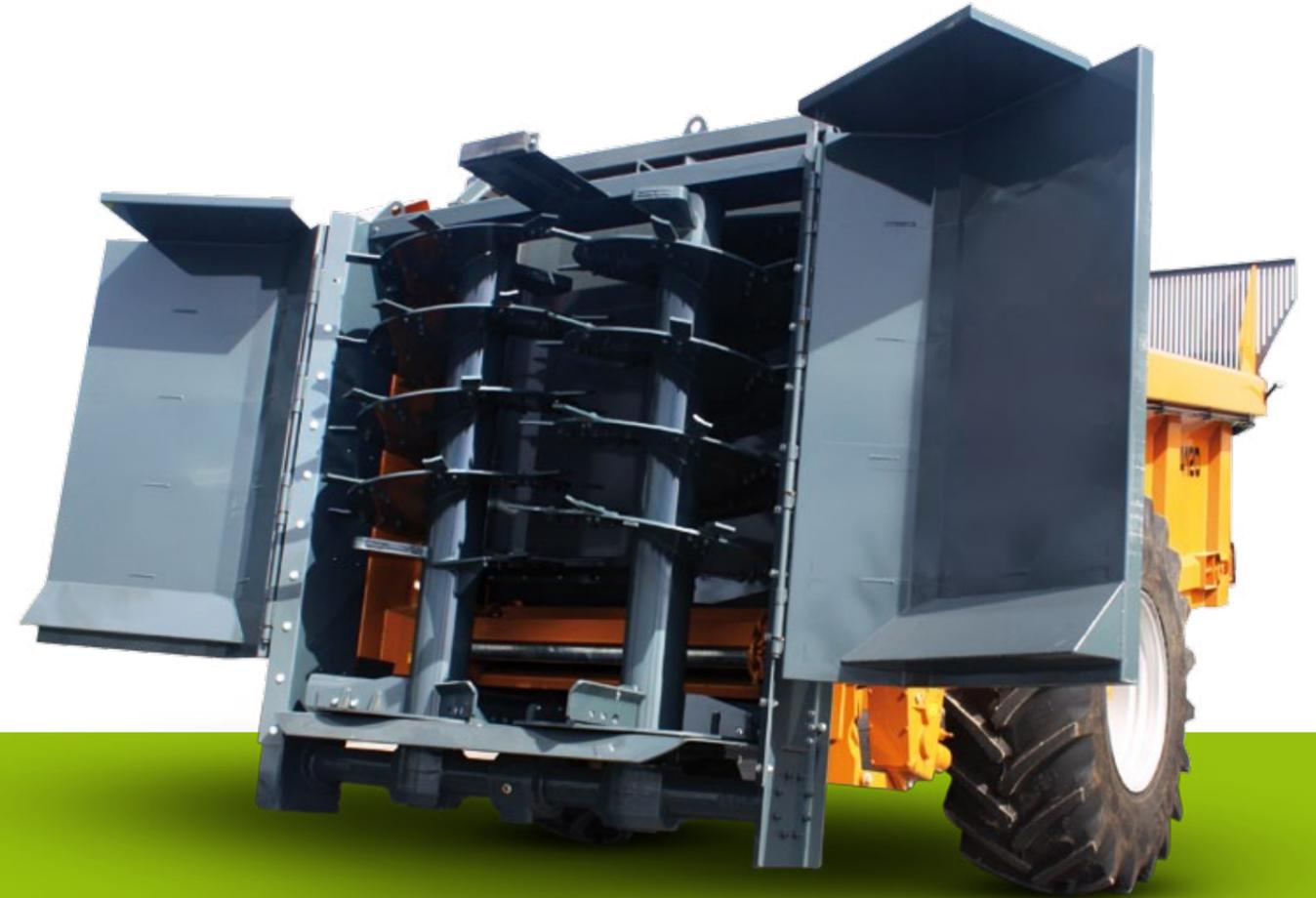
The new 1100mm diameter rotors have a disc base with three blades and replaceable wearing - parts. The option of a hydraulic folding canopy door allows the spreader to be used as a vertical beater spreader or with the doors closed the spreader can be used as a spinning disc spreader. The large diameter rotors are fitted as standard on the D4120 and D4150 and optional on the D4100.
