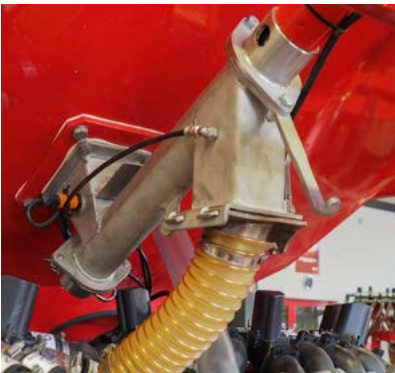
Micro-granules metered by an auger (Sprinter 3/4/6 ST)
