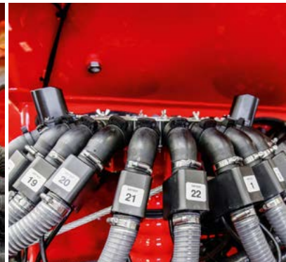
Permanent seed flow control by means of sophisticated sensor technology (optional)
