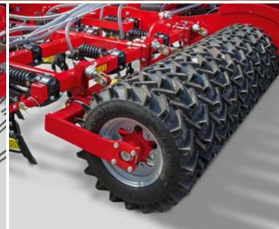
Front packer for first levelling and then improved depth control
