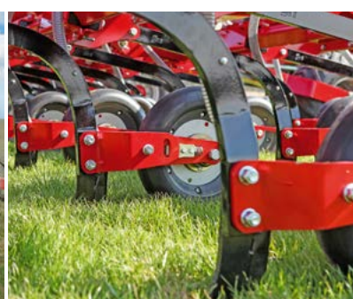
NT chisel coulters remove lumps from the seed horizon and place the grain precisely
