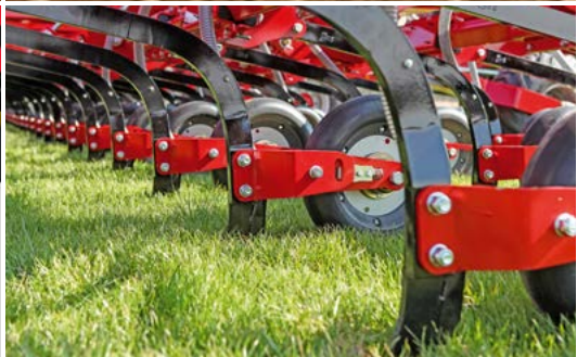
NT chisel coulters remove lumps from the seed horizon and place the grain precisely
