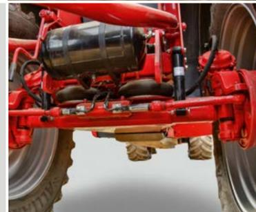
High clearance and smooth underbody with spring-loaded axle, optional: pneumatic suspension
