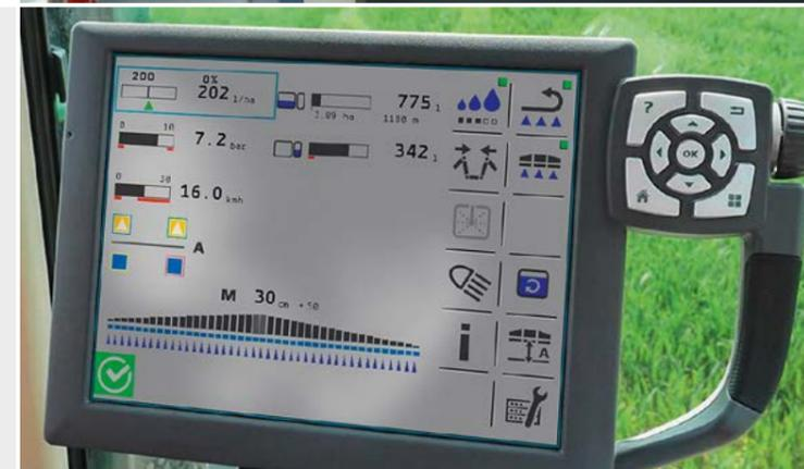
The Leeb GS can be controlled via various external terminals and joystick or the multifunction controller of the tractor.
