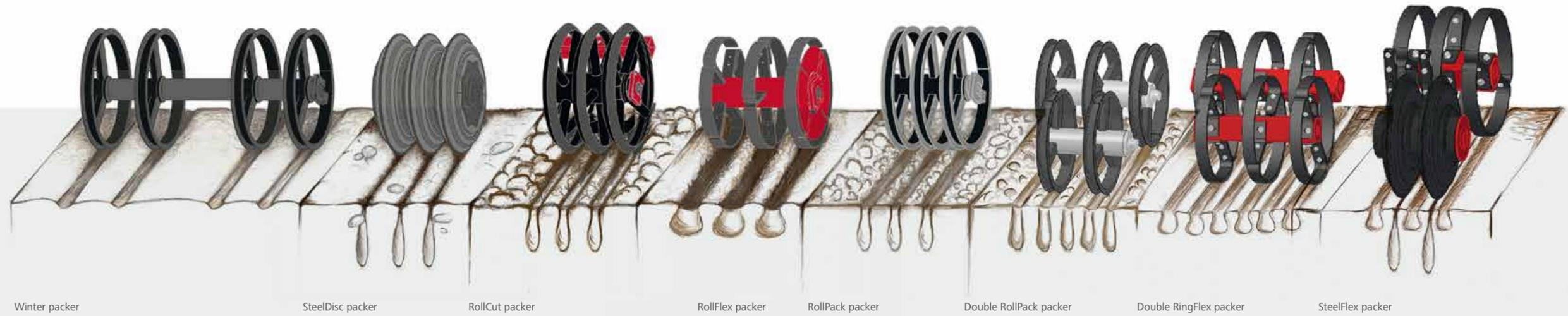
HORSCH can supply the appropriate packer version for deep as well as for shallow consolidation. The choice of the packer depends on the soil and HORSCH has a reasonable solution for any type of soil. Due to the consolidation excessively loose soil is compacted, clods are destroyed and an ideal environment with an optimum ratio of water- and air-bearing pores is created.
