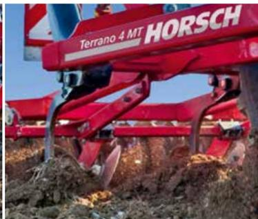
**TerraGrip tines with LD points** for deep loosening of the soil
