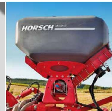
MiniDrill with a hopper capacity of 400 litres
