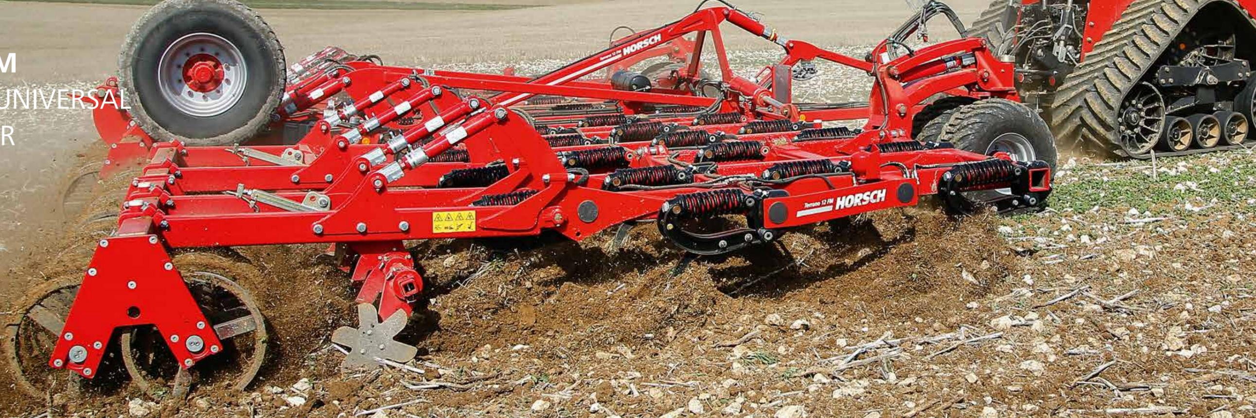
The **Terrano FM** is ideal for shallow stubble cultivation and medium-deep tillage, depending on the tractor power. Due to its 4-bar design it achieves intensive mixing and with a tine spacing of 27 cm the horsepower requirement is still low.
