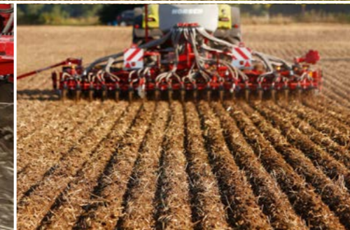
TurboDisc seed coulters place the seed into lump and residue-free soil.
