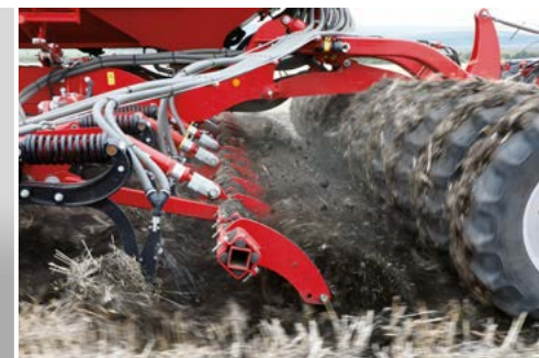
Crumbling tool Produces additional fine earth in the sowing area
