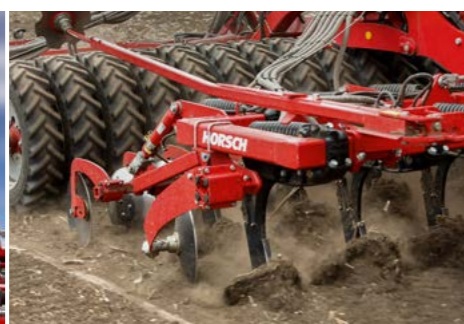
TerraGrip tines run exactly in front of the tyres
