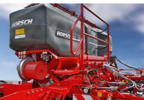
Ladder to guarantee safe access to the hopper openings
