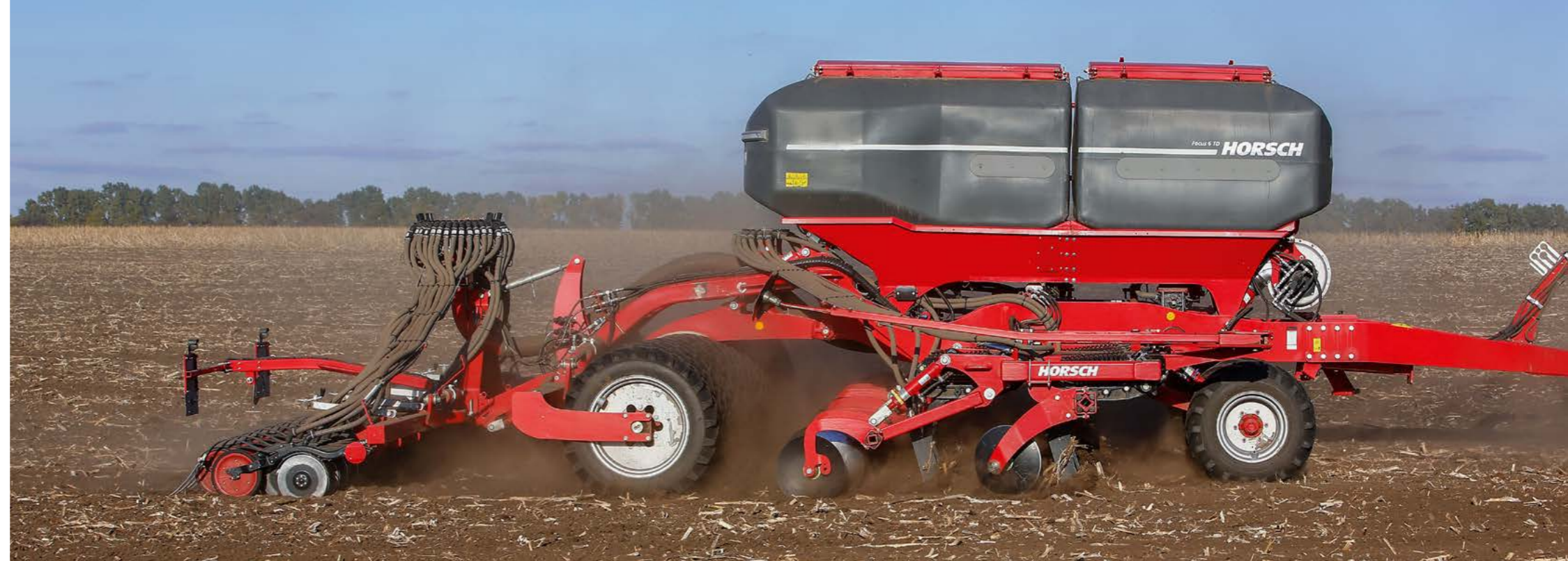
The four areas of the Focus TD TurboDisc seed coulters – hollow levelling discs – tyre packer – TerraGrip tines with LD points
