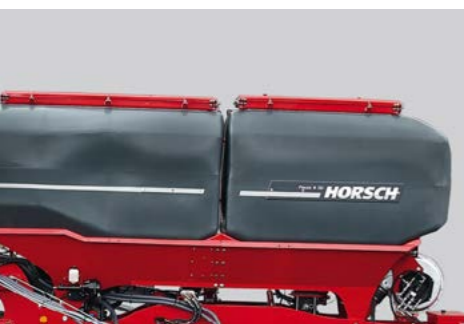
5 000 litre hopper (Partition: 2 000 litres front – 3 000 litres rear)
