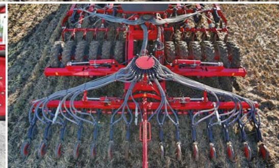
Sowing rape with row spacings of 28.6–30, 35 and 50 cm, optionally with TurboDisc or TurboEdge coultter
