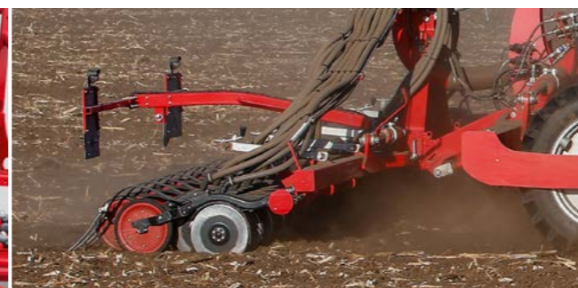
The above-average flexibility (15 cm) of the TurboDisc coulters with integrated press wheel allows for a precise and even depth control. The high individual coulters pressure of up to 120 kg guarantees smooth operation even at speeds above 12 km/h.
