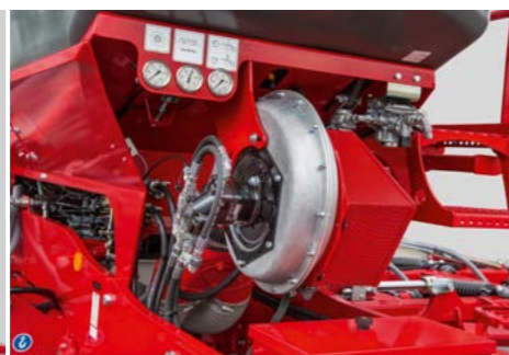
Hydraulic fan Direct drive and well-arranged cable set
