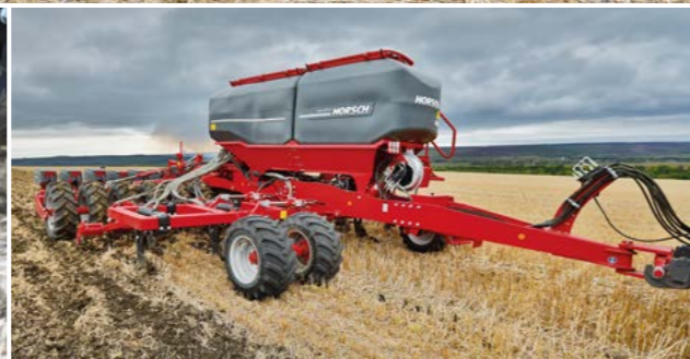
Row spacing of 50 cm, tyre packer runs exactly between the loosening rows
