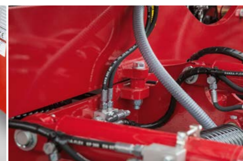
Attachment points for switching from tine to disc system. Simple replacement due to only 4 fixing points.
