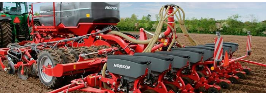
Focus TD with 3-point linkage and a Maestro RC seed unit bar
