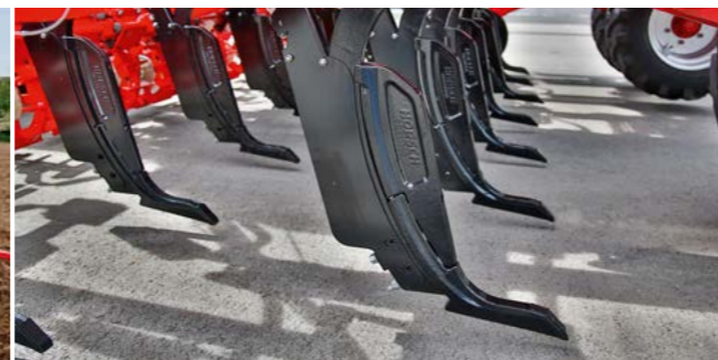
ULD+ points loosen the soil deeply and even in heavy soils, do not bring large clods to the surface.
