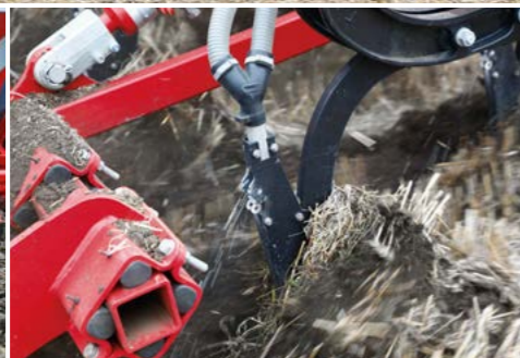
Targeted fertilisation in the row with the following option: deep, shallow or 50:50
