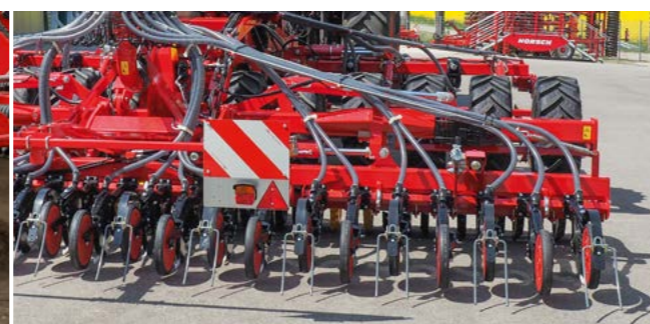
A TurboDisc coulters is placed in the middle behind a TerraGrip tine and a tyre
