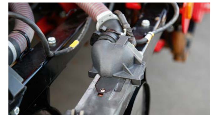
Bypass seeding system for seed rates beyond 250 grains/m 2 or seed that is not suitable for singulation
