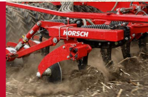
LD points cultivate the soil and place an exactly placed fertiliser deposit.
