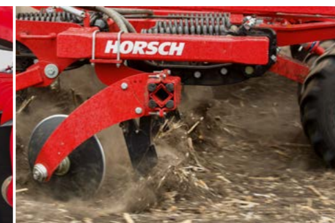
TerraGrip III L Release force 630 kg
