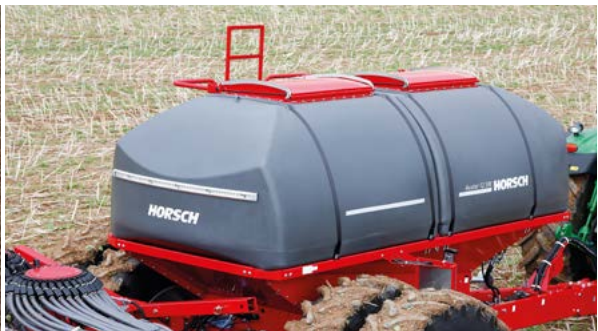
Capacity of 12 000 litre with a 50 : 50 split hoppers
