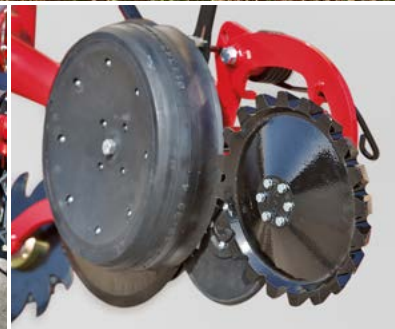
Star roller steel – excellent crumbling effect even in case of a high amount of organic substance
