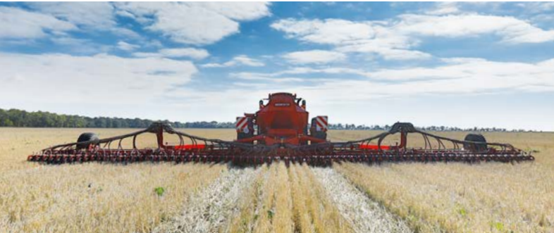
Hydraulic weight transfer from the seed waggon to the coulter frame: Regularly high coulter pressure over the whole working width.
