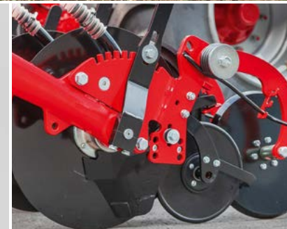
Fine adjustment of the sowing depth
