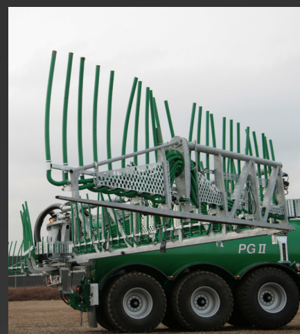
The new drip stop rotates the hoses so they point upwards.
