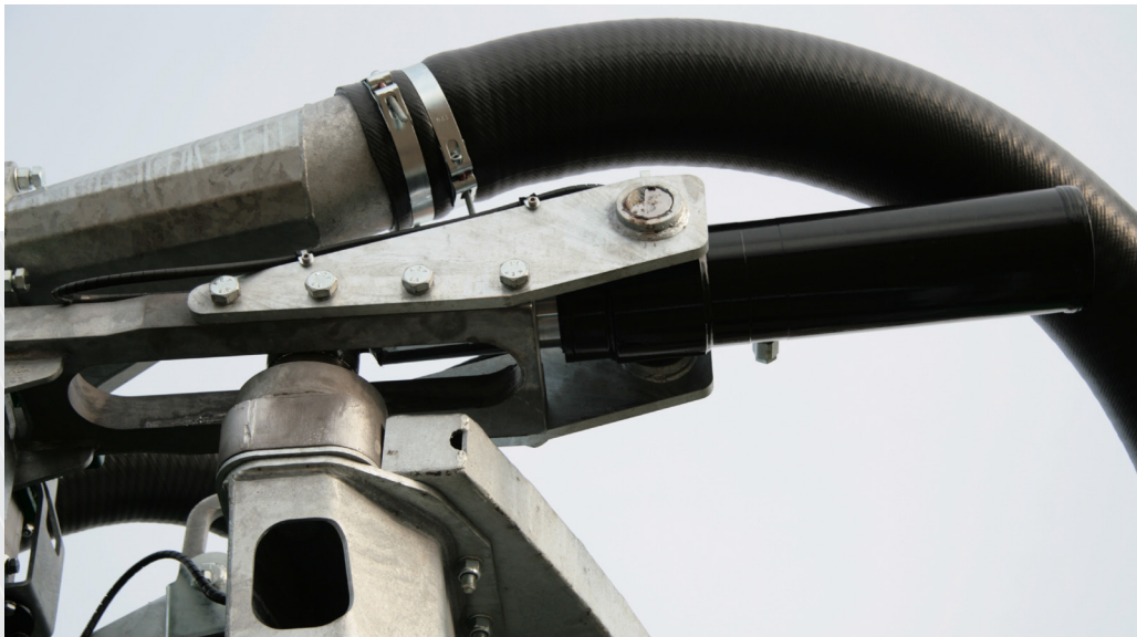
The two large side wings are hinged at the bottom and are held by a large cylinder at the top.
