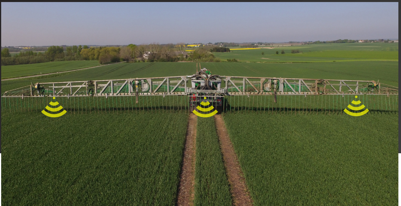
The height of the boom is monitored and adjusted via three ultrasonic sensors.
