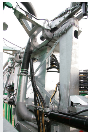
The boom has a simple central frame with no moving parts.
