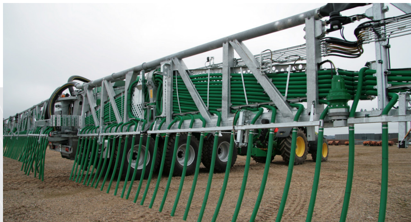
There are fewer "hose metres" in the new SHB4/36m drip hose boom.
