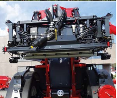
Boom middle section for working width ranging from 18 to 30 metre, optionally available with pivoted frame.
