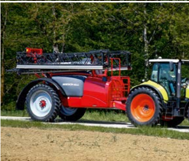
Boom does not reach to the front towards the tractor cabin
