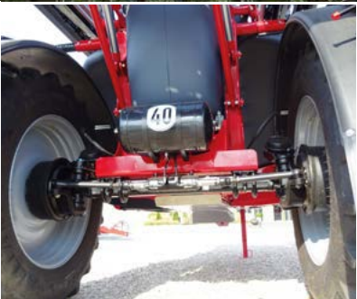
Three suspension versions are available: non-suspended, elastomer buffer and pneumatic suspension
