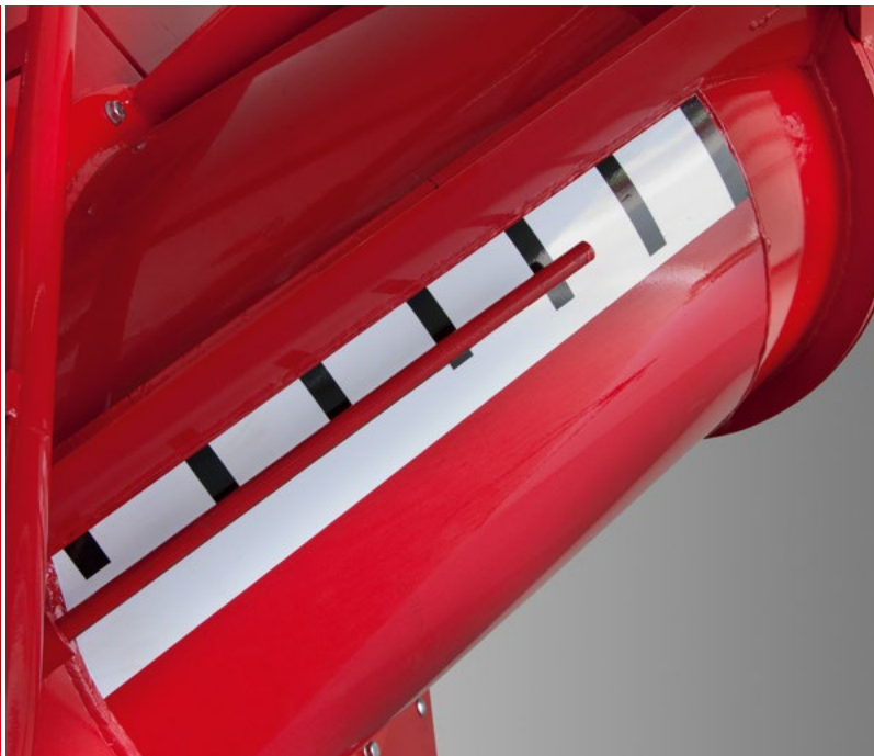
Display of the opening situation of the hydraulic slider in the auger waggon is clearly visible from the tractor cabin.
