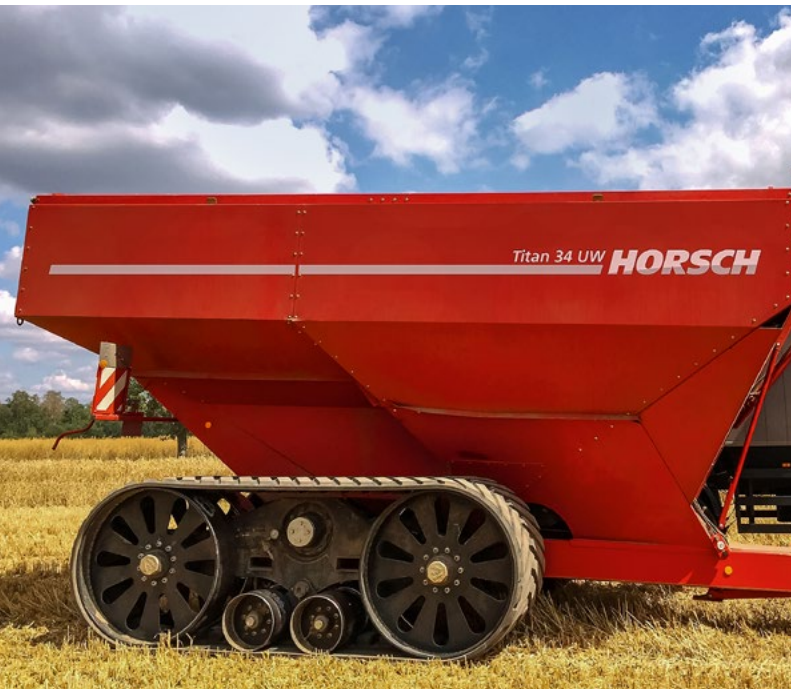
Due to the option of power tracks ground pressure is reduced (contact area 4.2 m²)
