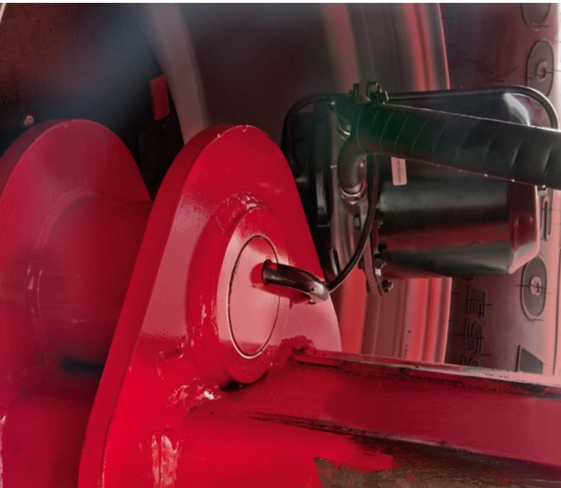
The wheel version of the auger wagon is available with a pneumatic brake. The power tracks can be equipped with a pneumatic or a hydraulic brake.
