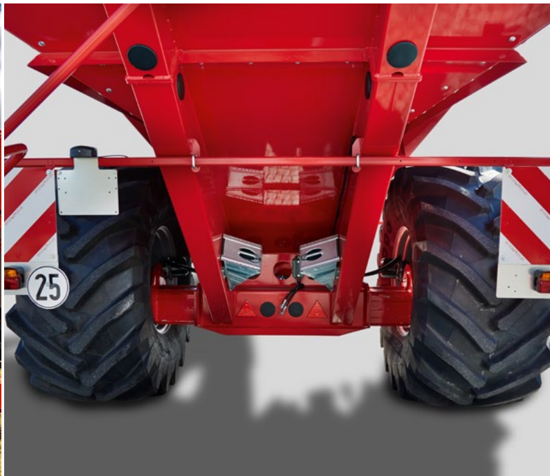
The telescopic rear axle increases the width from 3 to 3.56 meters and thus guarantees more soil-saving and stability.
