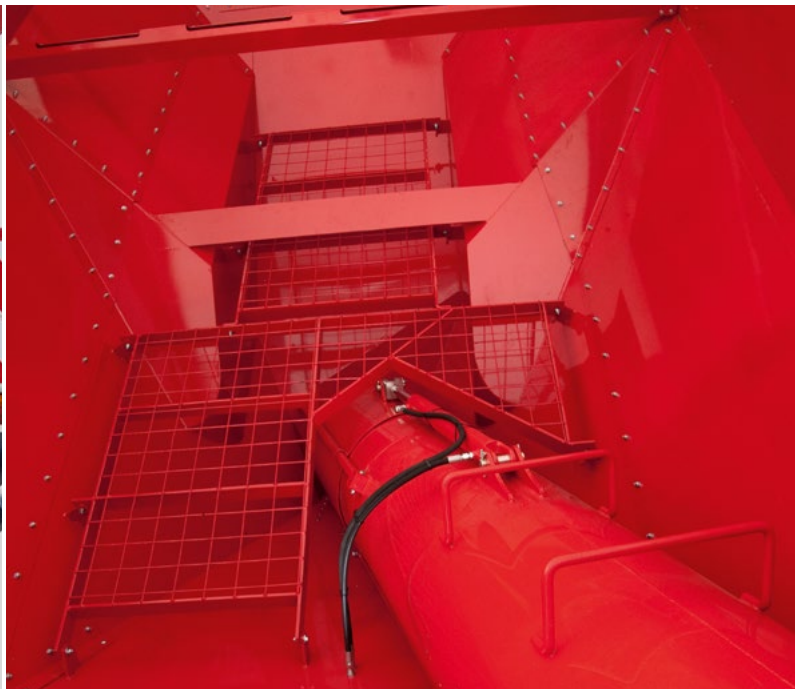
The inside of the complete hopper is easily accessible and walkable for easy cleaning.
