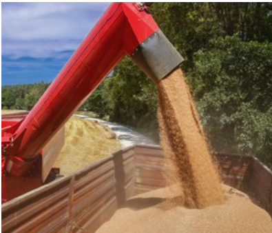
The output of the newly designed hydraulically foldable auger conveyor is 18 tons per minute – corresponding to gigantic 1 000 tons per hour.
