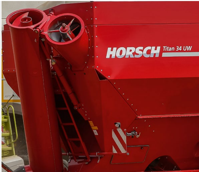
The output of the hydraulically foldable conveyor auger amounts to 18 tons per minute and, thus, the Titan UW is emptied in 90 seconds.
