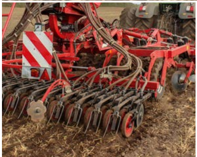
TurboDisc coulters 15 cm coulters spacing, integrated coulters suspension, variable coulters pressure of up to 120 kg/coulters
