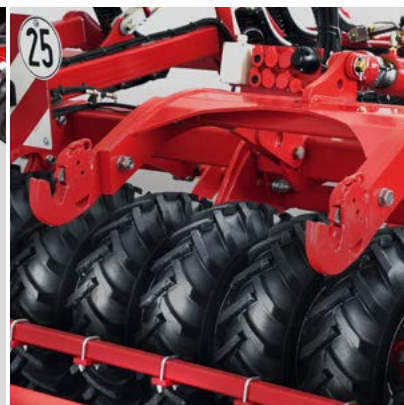
Two-point linkage with hydraulic and electric connections
