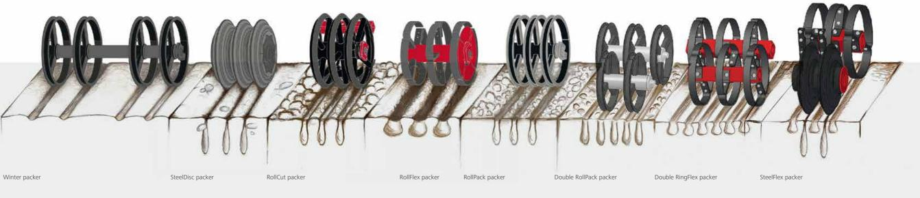
HORSCH can supply the appropriate packer version for deep as well as for shallow consolidation. The choice of the packer depends on the soil and HORSCH has a reasonable solution for any type of soil. Due to the consolidation excessively loose soil is compacted, clods are destroyed and an ideal environment with an optimum ratio of waterand air-bearing pores is created.
