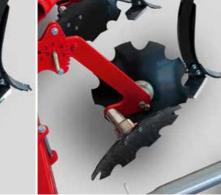
Spring-loaded levelling discs
