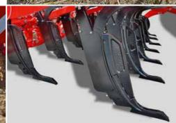
ULD+ points loosen the soil deeply and even in heavy soils, do not bring large clods to the surface.
