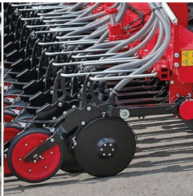
PowerDisc with parallelogram suspension
