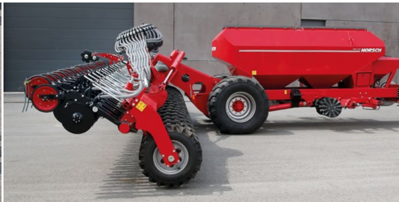
Chassis is only used for transport
