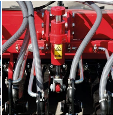
Coulter pressure adjustment hydraulically infinitely adjustable
