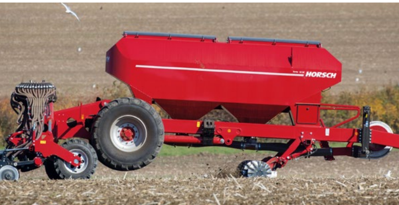
Divided pressurised hopper in the ratio 60 : 40 (3 600 l front & 2 400 l rear)
