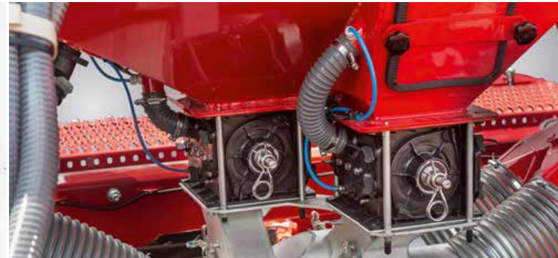
Two identical metering units Precise metering of seeds and fertiliser
