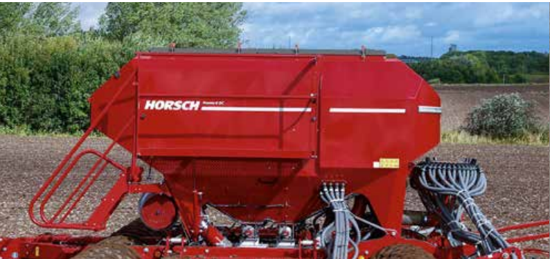
Large double hopper Hopper capacity up to 5 000 l, partition 40 : 60
