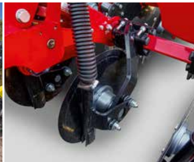
The fertiliser coulters of the HORSCH PPF system place the fertiliser at the exact depth to guarantee an optimum development of the seed grain.
