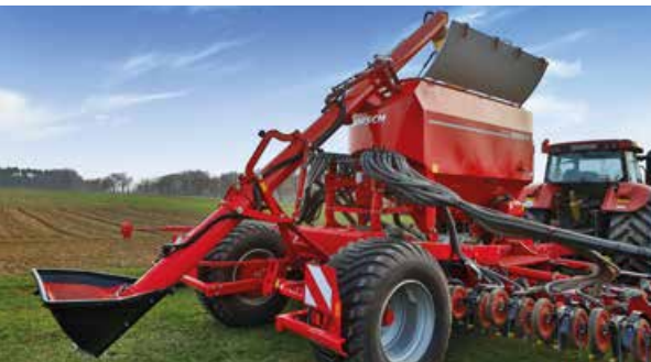
Filling auger double hopper output 500 kg/min
