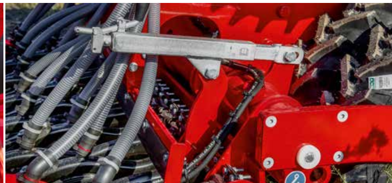
Stepless coulter pressure adjustment Manual adjustment increases the pre-load of the rubber elements
