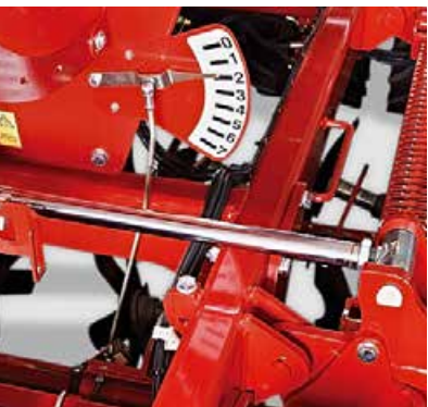
Easy working depth adjustment Hydraulic adjustability during operation
