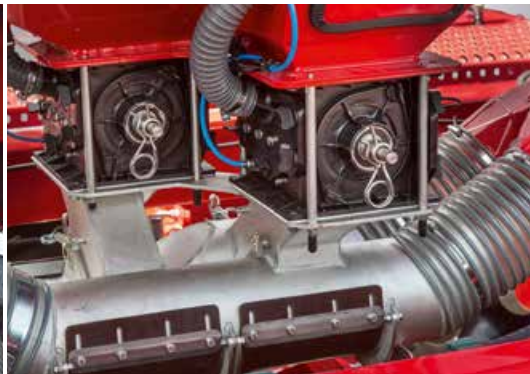
Double fall sluice for simultaneously applying fertiliser in one flow
