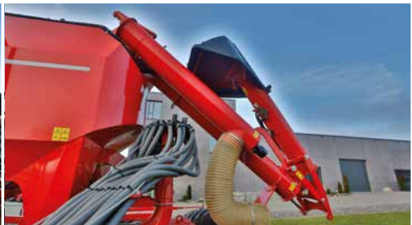
Hydraulically foldable in transport position
