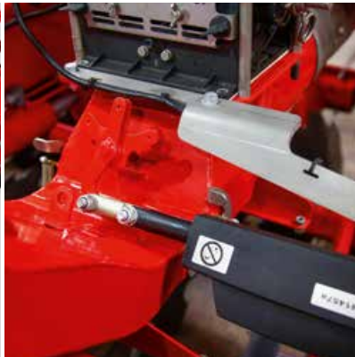
Half-width shut-off electr. Pronto 6 DC/AS
