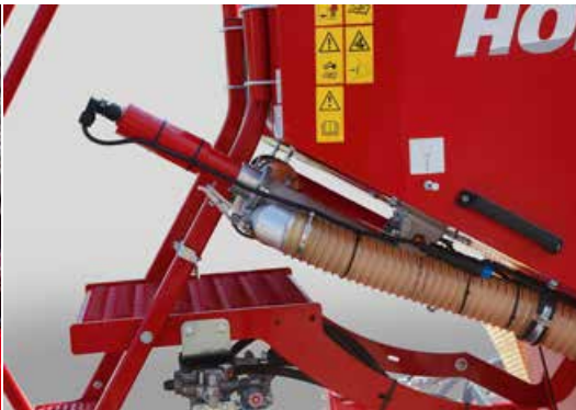
Micro-granular metering device Pronto 3–6 DC (single hopper)
