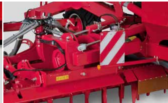
3 m segments of the rotary harrow are oscillatingly suspended for an optimum soil adjustment.
