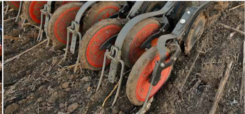
Double disc coulter Straight discs with inner maintenance-free bearings
