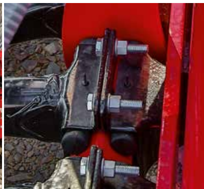
Shock absorbed mounting Good contour-following capability and overload protection
