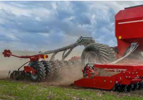
Transport system Pronto AS Large tyres (800/40–26.5), low draft requirement and reduced soil pressure
