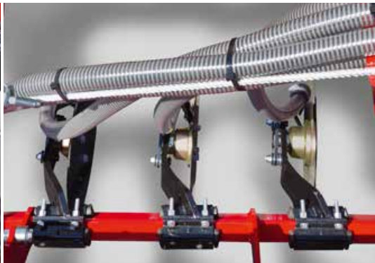
Variable depth adjustment Fertiliser placement between two seed rows, in the centre line of the tyre
