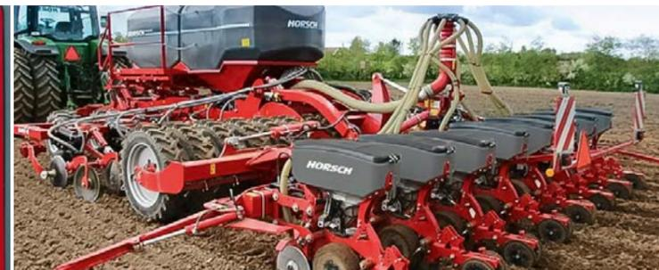
Focus TD with 3-point linkage and a Maestro RC seed unit bar
