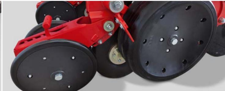
Depth control wheels with scraper, adjustable press wheels and the catching roller which can be removed in extremely wet conditions as the seed grain is not placed into the soil with pressure
