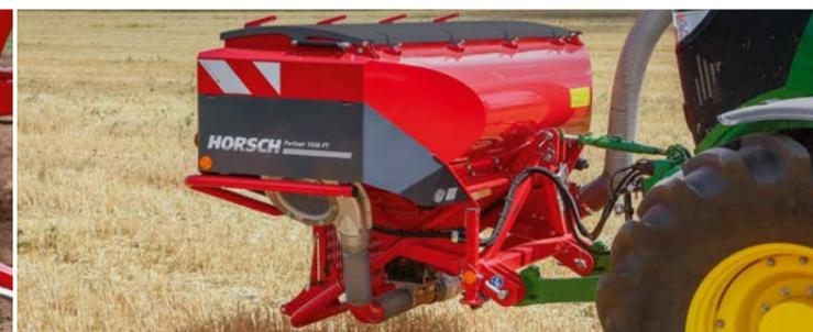
The Partner FT with a hopper capacity of 1 600 litres can be combined with the Maestro RC in an optimum way
