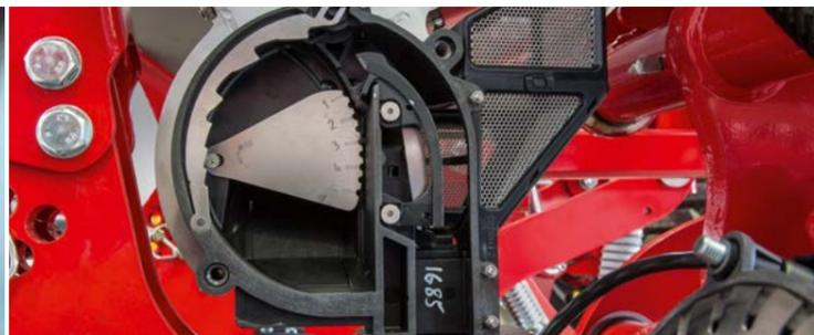
The adjustable **scraper** transports the grain into the fall sluice without any disturbing centrifugal forces
