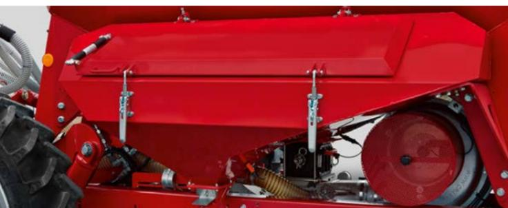
Hopper micro-granular unit **Maestro CC** (200 litre), 12/18 **SW** (350 litre) and 16/24/36 **SW** (500 litre) with placement in the seed furrow
