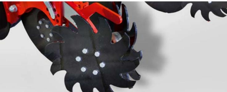
Optional **trash wheels** in front of the fertiliser coulters
