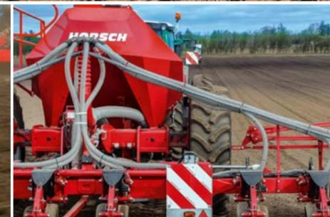
**Seed waggon** for 2 000 litre seed and 7 000 litre fertiliser for maximum efficiency
