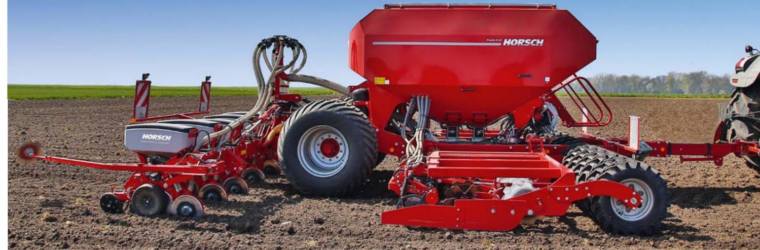
**Maestro RC:** Maestro seed bar (8- or 12-row) combined with seed wagon of the Pronto AS. The Pronto seedbar can be replaced with the Maestro seedbar and vice versa via a 3-point.
