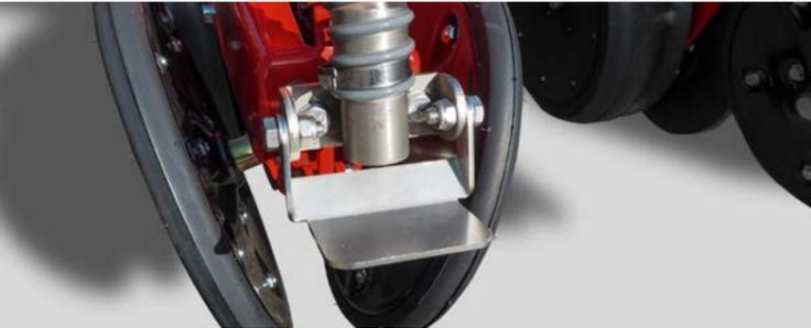
Outlet micro-granular compound for slug pellets
