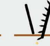
The spiked and the finger press wheels version breaks the consolidation that was generated by the depth control wheels.
