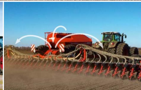
Transfer of the seed waggon weight to the seed bar for increased coulter pressure
