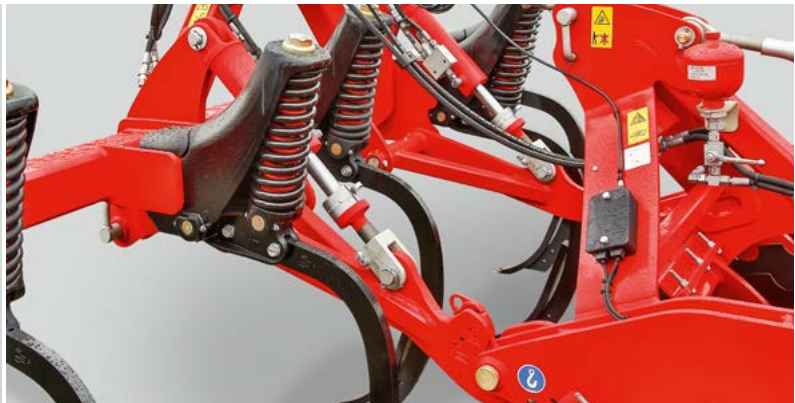
Mono TG: Ideal for deep loosening. TerraGrip tines with narrow LD (low disturbance) coulter deeply loosen soil without transporting rough lumps to the surface.
