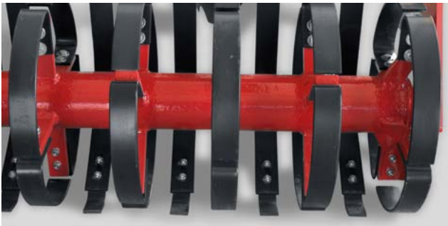
Levelling tines between packer rings ensure good levelling of soil surface
