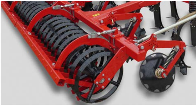
RollCut packer good surface structure on medium-heavy soils without stones
