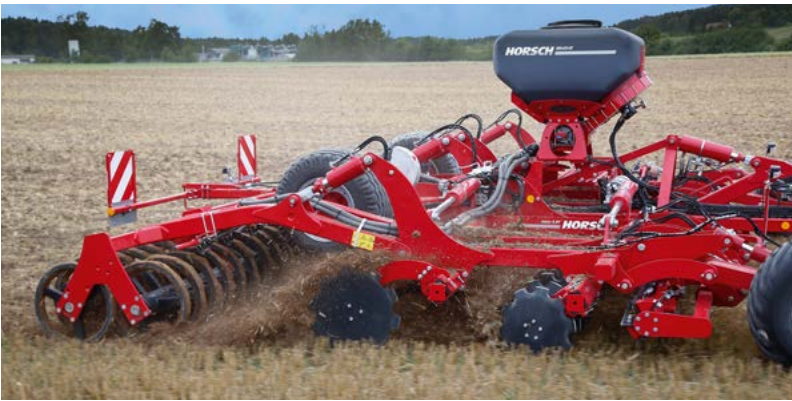
Joker RT with optional MiniDrill: Seed distribution in front of the packer by means of a deflector plate
