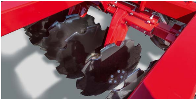
Large (Ø 62 cm) discs for working deeply
