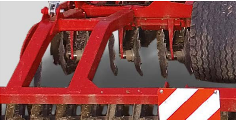
High clearance – two discs at one arm
