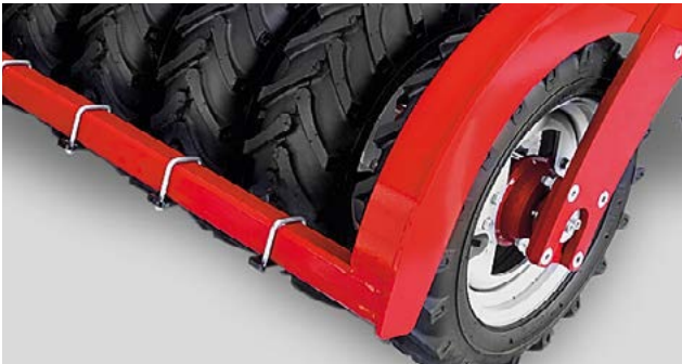
Flexible tyre packer with tires with AS-profile
