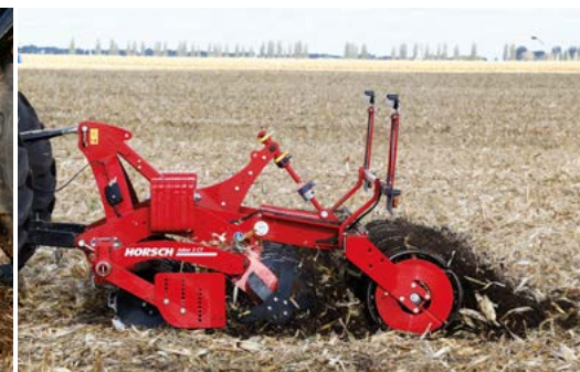
Optimum clearance clearance due to arrangement of the discs in pairs
