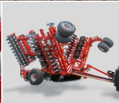
Joker 10/12 RT Compact transport dimensions; 3 m transport width, 4 m transport height
