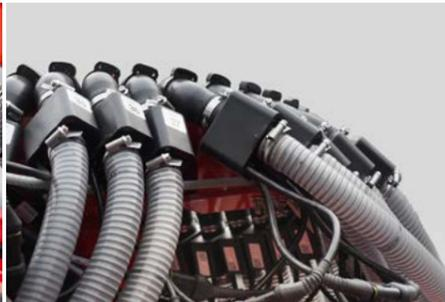
**Solid monitoring sensors** for seed and fertiliser
