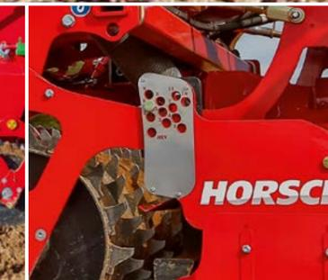
Simple and easily understandable adjustment of the working depth of the rotary harrows
