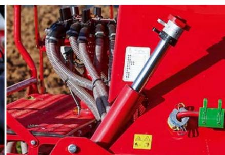
**Hydraulic sowing depth adjustment with clips**
