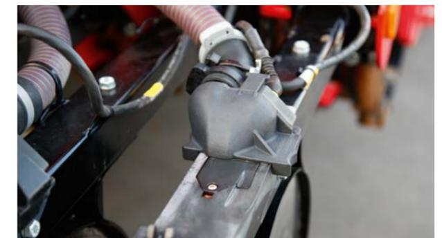
Bypass system for seed rates beyond 250 grains/m<sup>2</sup> or seed that is not suitable for singulation
