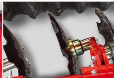
**2-row DiscSystem** – Considerably lower horsepower requirement compared to powered front tools (e. g. power harrow). Excellent seedbed preparation at high working speeds
