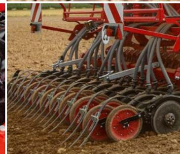
TurboDisc precision coulters of the second generation for exact seed placement even at high operational speed. In all Express TD and KR.
