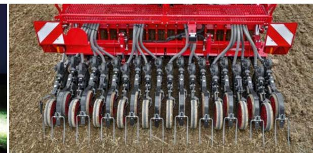
Optimum arrangement of the **seed coulters** behind the strip packer. One seed coulters runs exactly in the strip that has been consolidated.
