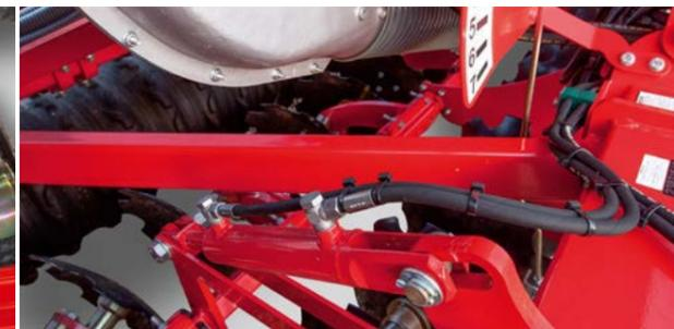
**Hydraulic depth adjustment DiscSystem** (optional)
