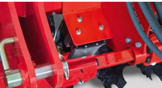
**Radar sensor** for an exact recording of the speed and to control the seed quantity
