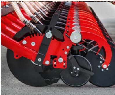
Press wheel in the seed furrow for optimum seed-soil contact of the grain
