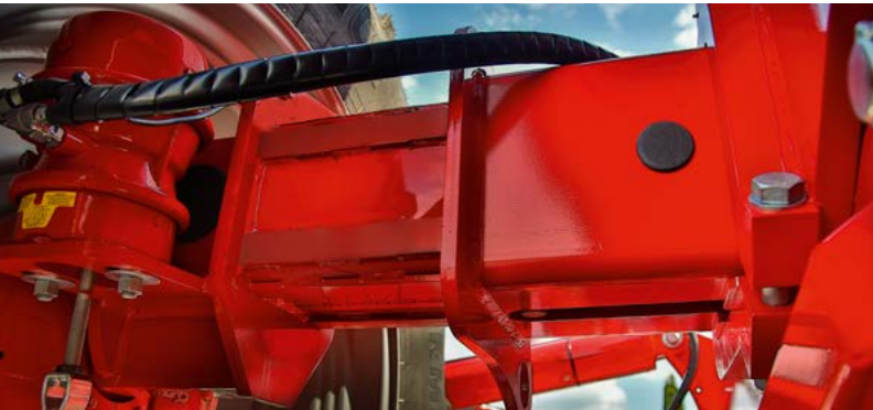
Standard telescopic axle Compact transport width; reduction of the track pressure behind the tractor track
