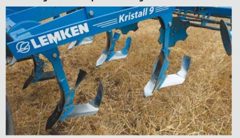
With its groundbreaking shape the newly developed TriMix share, with its curved guide plates on the wing shares, provides an unprecedented level of mixing in comparison with all wing shapes previously offered.
