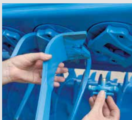
Replacing a quick-change tine
