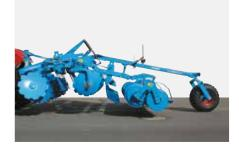
The semi-mounted system with transport wheel
