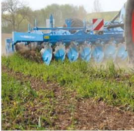
Compact disc harrows provided previously intense and homogeneous mixing of soil and organic matter to a depth of approximately 12 cm.
