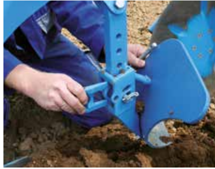
Adjustment of the skimmers without tools
