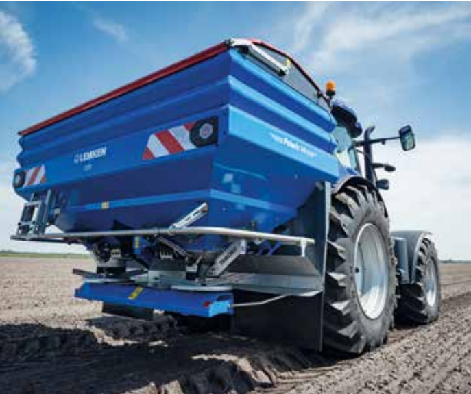
Hydraulic drive for constant disc speeds even on slopes
