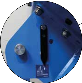
Angle adjustment and display for precise late top dressing
