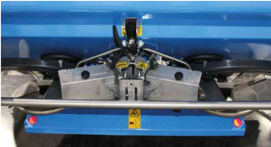
Hydraulically lowerable border deflector for spreading across half working widths
