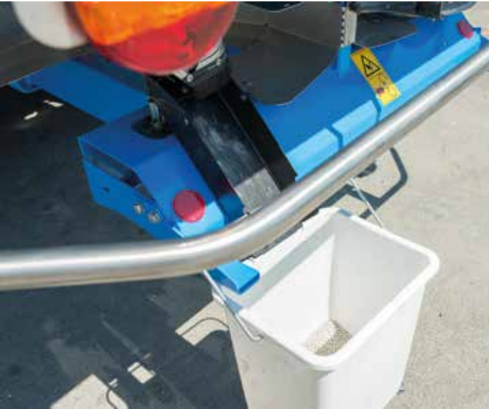
Calibration test kit comprising a feeder chute, bucket and adjustment shutter
